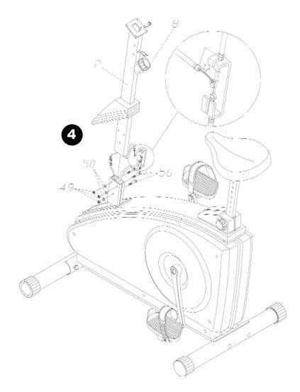
**4.** Slide the console tube (2) through the console tube collar (14, 15). Connect the computer cable in the console tube to the computer cable in the main frame. Attach the console tube (2) to the frame with the locknuts (49), flat washers (50) and screws (56) provided. Attach the console tube collar (14, 15) to the main frame (1) with screws (57).
